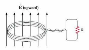
(a) Find the induced emf produced in the coil during the time interval of 4 s.
